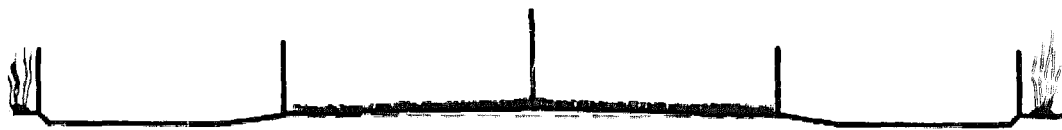
(b). Pegging and digging side drains.
